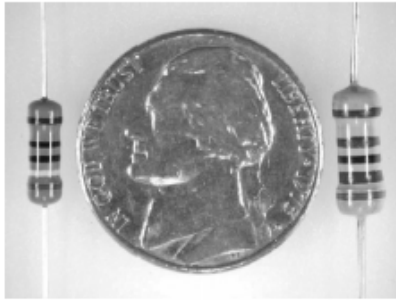
Figure 1.43 Typical 1/2-W resistors ( Jim Kearns )
