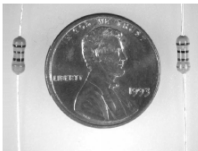
Figure 1.42 Typical \frac{1}{4} -W resistors ( Jim Kearns )
