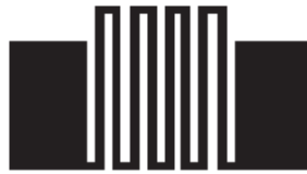
Figure 1.64 Metal-foil resistance strain gauge
