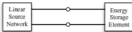
Figure 4.16 Generalized first-order circuit seen as a source network attached to an energy storage element as the load
